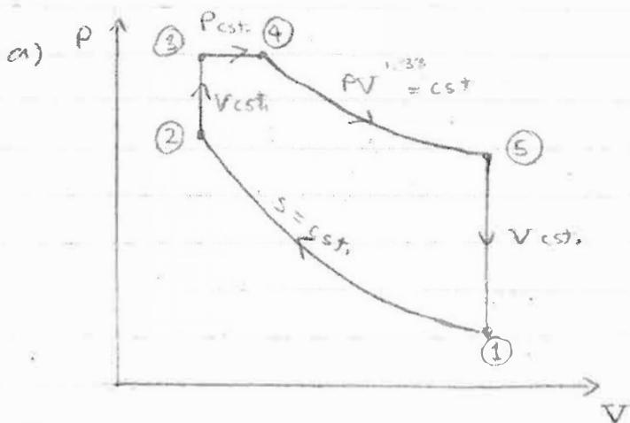
b) ①  $P_1 = 100 \text{ kPa}$  :  $V_1 = \frac{mRT_1}{P_1} = \frac{(0.002)(0.287)(300)}{100}$
