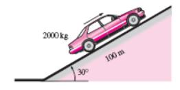
$$\dot{W}_g = mg(z_2 - z_1) / \Delta t = (2000 \text{ kg})(9.81 \text{ m/s}^2)(50 \text{ m}) \left(\frac{1 \text{ kJ}}{1000 \text{ kg} \cdot \text{m}^2/\text{s}^2}\right) / (10 \text{ s}) = 98.1 \text{ kW}$$
