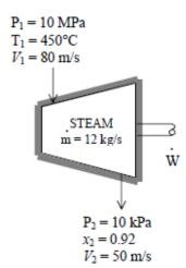
Assumptions 1 This is a steady-flow process since there is no change with time. 2 Kinetic and potential energy changes are negligible. 3 There are no work interactions. 4 The device is adiabatic and thus heat transfer is negligible.
