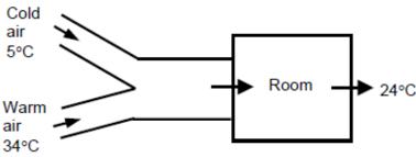
Analysis (a) We take the mixing chamber as the system, which is a control volume since mass crosses the boundary. The mass and energy balances for this steady-flow system can be expressed in the rate form as
