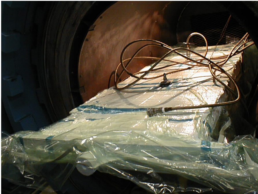
6-cell bridge wrapped in vacuum bag ready for curing in autoclave
