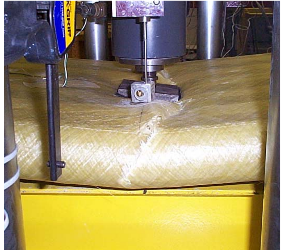
Local buckling of fibers in compression (top surface)
