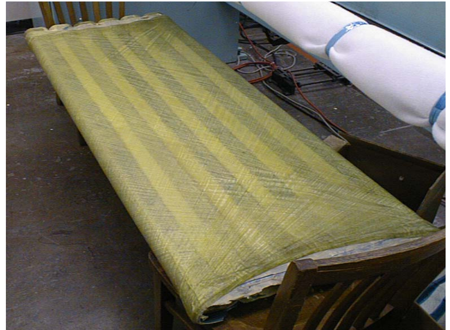
Final 6-cell bridge structure
