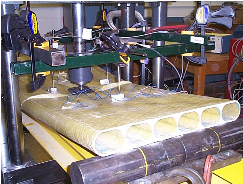
Failure of outer shell at 7.7 kips (max. load carried by structure)
