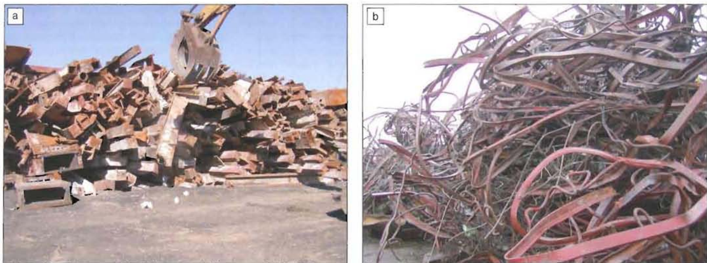
Figure 4. (a) Core columns, perimeter columns, and beams from the Twin Towers in a salvage yard in New Jersey. Critical pieces for the NIST investigation were recovered here. (b) Typical condition of the floor trusses in the salvage yards. The lightweight trusses were severely damaged during the collapse. Furthermore, since bridging trusses had been welded to the main trusses in a full-floor cross-grid system, the trusses had to be cut up and compacted in order to remove them from the collapse site.
