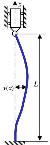
$$\begin{pmatrix} v(0) \\ \phi(0) \\ v(L) \\ \frac{M(L)}{EI} \end{pmatrix} = \begin{pmatrix} 1 & 0 & 0 & 1 \\ 0 & 1 & n & 0 \\ 1 & L & \sin(nL) & \cos(nL) \\ 0 & 0 & n^2 \sin(nL) & n^2 \cos(nL) \end{pmatrix} \begin{pmatrix} C_1 \\ C_2 \\ C_3 \\ C_4 \end{pmatrix} = \begin{pmatrix} 0 \\ 0 \\ 0 \\ 0 \end{pmatrix}$$
