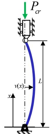
$$\begin{pmatrix} v(0) \\ M(0)/E I \\ v(L) \\ M(L)/E I \end{pmatrix} = \begin{pmatrix} 0 \\ 0 \\ 0 \\ 0 \end{pmatrix} = \begin{pmatrix} 1 & 0 & 0 & 1 \\ 0 & 0 & 0 & -n^2 \\ 1 & L & \sin(nL) & \cos(nL) \\ 0 & 0 & -n^2 \sin(nL) & -n^2 \cos(nL) \end{pmatrix} \begin{pmatrix} C_1 \\ C_2 \\ C_3 \\ C_4 \end{pmatrix}$$
