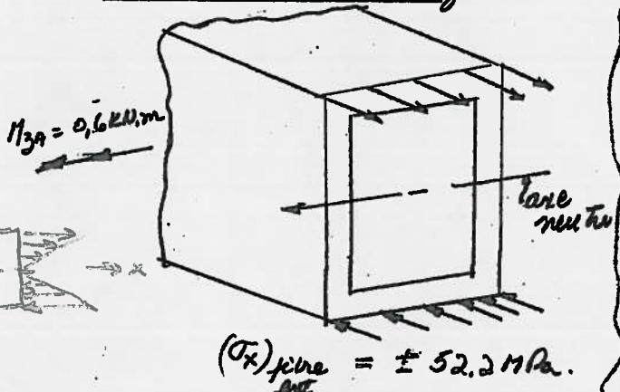
$$(\sigma_x)_{\text{fibre ext.}} = \pm 52,2 \text{ MPa.}$$
