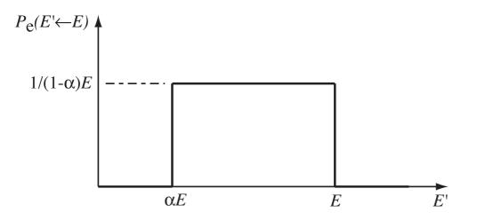
The probability density is uniform in the support  $\alpha E \leq E' \leq E$ . The collision of a neutron on a nucleus initially at rest has the effect to slow down this neutron. The slowing-down effect is more important for light nuclides, as they are characterized by small values of  $\alpha$ .
