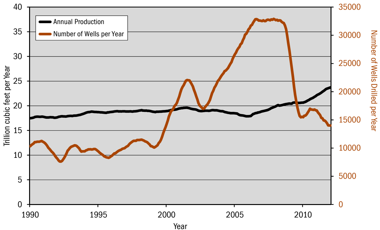
Figure 20. U.S. natural gas production versus annual drilling rate of successful gas wells, 1990-2012. 27
