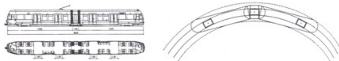
(a) 6-axle 70% low floor 28.40 m long car for Cologne, Croydon, Stockholm and Istanbul
