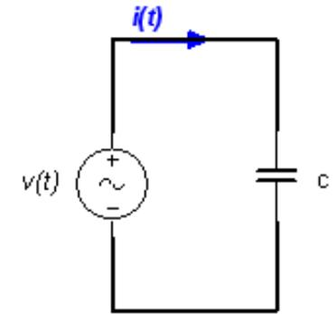
$$\Rightarrow i(t) = \underbrace{C\omega V_{\max}}_{I_{\max}} \cos\left(\omega t + \underbrace{\theta_v + \pi - \frac{\pi}{2}}_{\theta_i}\right) \Rightarrow \begin{cases} I_{\max} = C\omega V_{\max} \\ \theta_i = \theta_v + \frac{\pi}{2} \end{cases} \Rightarrow \varphi_C = -\frac{\pi}{2} \Rightarrow FP_C = 0 \text{ avance}$$
