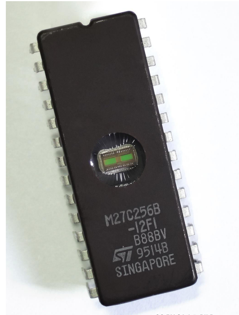
EPROM 32 KB, STMicroelectronics M27C256B
