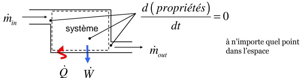
$$\dot{E}_{sys} \equiv \frac{dE_{sys}}{dt} = 0, \dot{m}_{sys} \equiv \frac{dm_{sys}}{dt} = 0 \text{ et } \frac{dV_{sys}}{dt} = 0 \text{ (travail PdV=0)}$$
