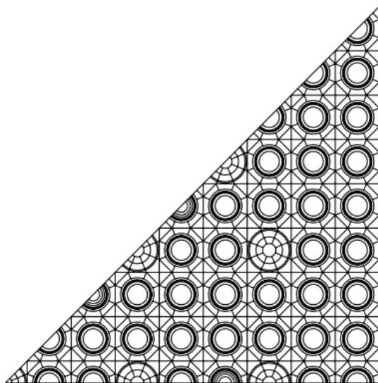
**Figure 3:** Geometry of an eight-symmetry PWR assembly with a water blade.
