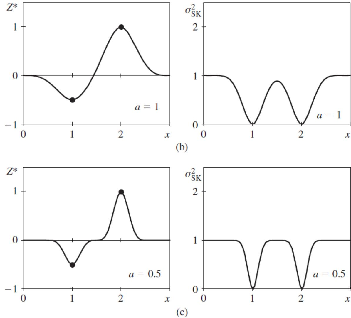
FIGURE 3.1 Simple kriging estimate and variance for the case of two data points and a cubic covariance model with  $C(0)=1$ . From (a) to (c): the estimator becomes “wigglier” as the range  $a$  decreases.
