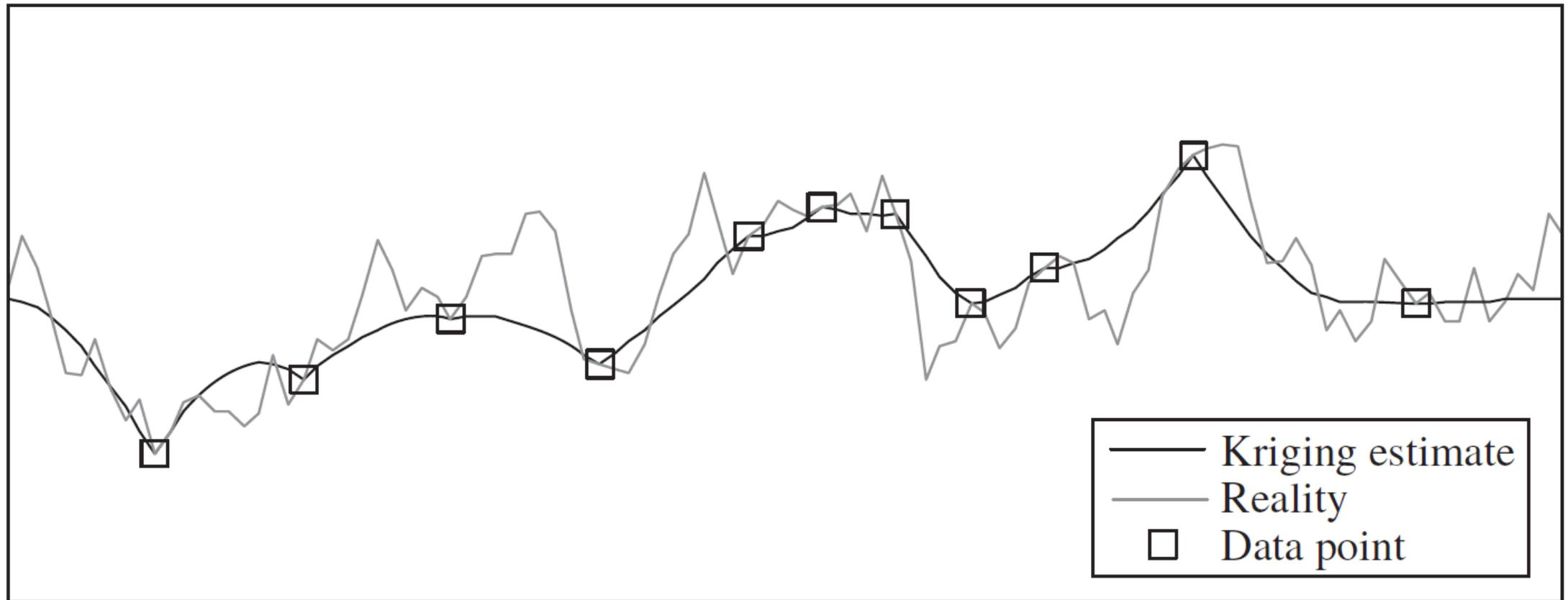
**FIGURE 3.2** Illustration of the smoothing effect of kriging.
