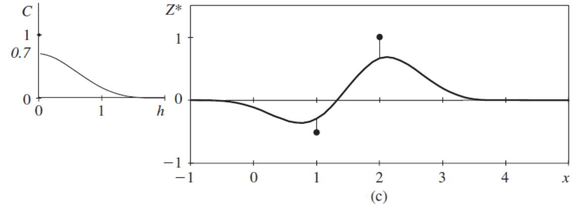
FIGURE 3.3 The dependence of the simple kriging estimate on the regularity near the origin of the covariance function: (a) parabolic behavior; (b) linear behavior; (c) discontinuity.
