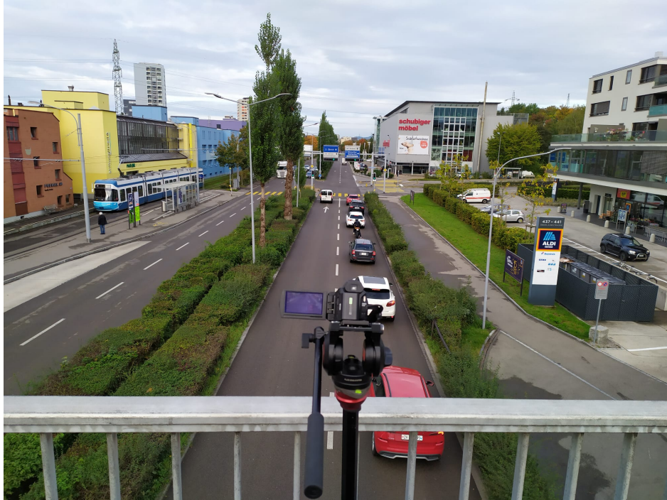
Figure 1: Example of camera setup on an overpass
