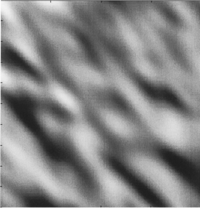
Figure 3. Two-dimensional anisotropic Gaussian random field with Gaussian covariance (grid: 200 \times 200 nodes; space step: 1; major correlation length: 50; minor correlation length: 20; mean: 0; variance: 1).
