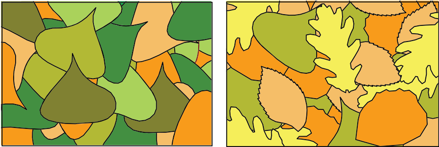
FIGURE 7.32 Realizations of mosaic random functions derived from dead-leaves models: (a) single-dead-leaves model (black poplar) with independent assignment of a value to each leaf; (b) multi-dead-leaves model with value assignment depending on leaf species (alder, elm, oak, poplar).
