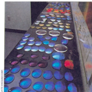
Interference effects cause residual reflected-light color, which can be a striking feature of thin-film coated eyeglass lenses.
