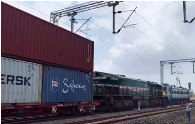
Figure 1. (Color online) Double-Stack Train Operations Under High-Rise Overhead Electric Line in Indian Railways (Press Information Bureau 2020)
