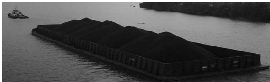
Figure 2: Coal transport operations utilize barges that carry between 3,000 and 10,000 tonnes of coal.
