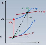
$$\frac{T_2}{T_1} = \left(\frac{p_2}{p_1}\right)^{\frac{R}{c_p\eta_p}}$$
