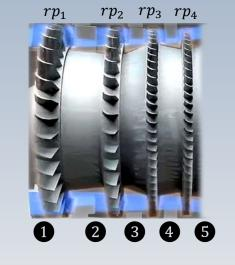
$$T_2/T_1 = \left(\frac{(rp_1)^{(\gamma-1)/\gamma} - 1}{\eta_{1s}}\right) + 1$$
