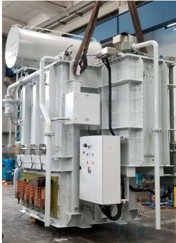
Figure 24.15 – Electrolysis Transformer FAT Test
