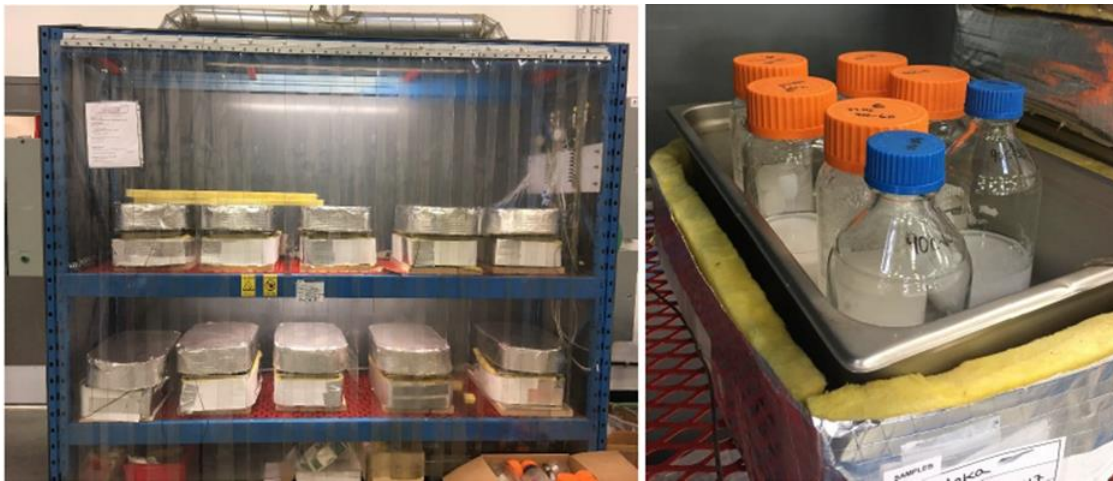
Figure 13.17 – Material Testing Rig for Solubility Tests at BCRI
