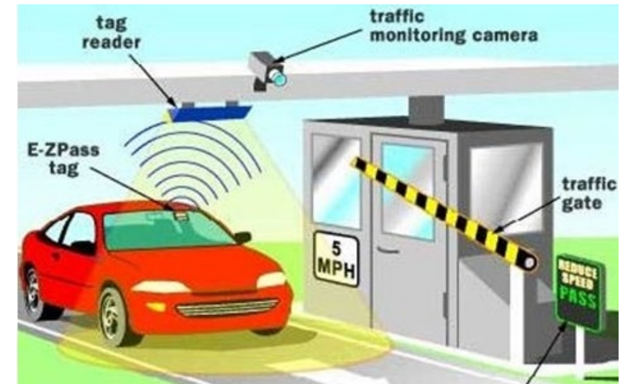
Electronic toll collection system
