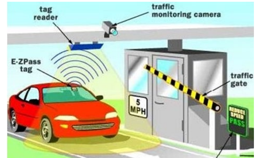
Electronic toll collection system
