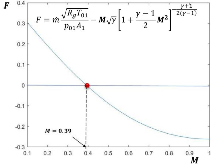
$$\dot{m} \frac{\sqrt{R_g T_{01}}}{p_{01} A_1} = M \sqrt{\gamma} \left[ 1 + \frac{\gamma - 1}{2} M^2 \right]^{\frac{\gamma + 1}{2(\gamma - 1)}}$$
