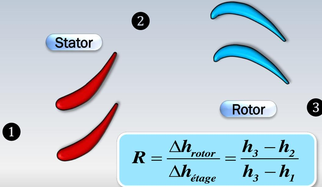
$$R = \frac{\Delta h_{\text{rotor}}}{\Delta h_{\text{étage}}} = \frac{h_3 - h_2}{h_3 - h_1}$$
