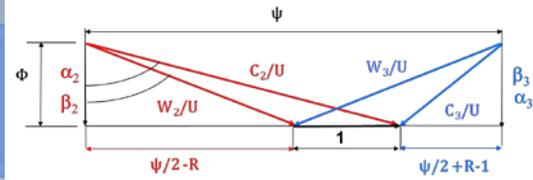
$$W_e = U(c_{3u} - c_{2u}) = U(c_{3u} + |c_{2u}|) = 2Uc_2 \sin \alpha_2$$
