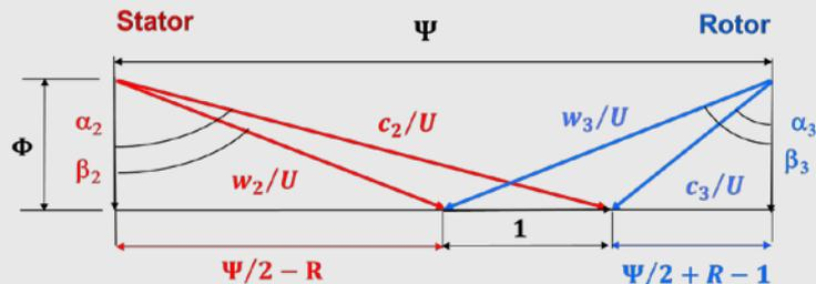
$$c_1 = \left( \frac{c_{1x}}{\cos \alpha_1} \right) = \left( \frac{\phi U}{\cos \alpha_1} \right) \quad \text{Étage répétitif} \quad (\alpha_1 = \alpha_3)$$
