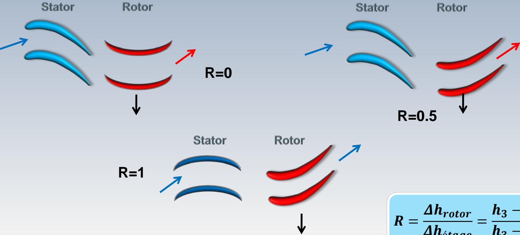
$$R = \frac{\Delta h_{\text{rotor}}}{\Delta h_{\text{étage}}} = \frac{h_3 - h_2}{h_3 - h_1}$$
