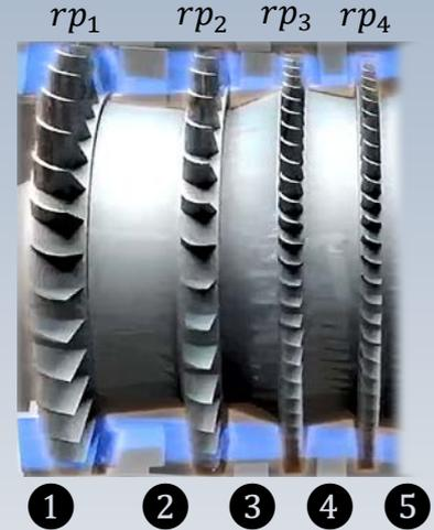
$$\textcircled{1} \quad T_2/T_1 = \left( \frac{(rp_1)^{(\gamma-1)/\gamma} - 1}{\eta_{1s}} \right) + 1$$
