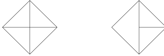
Fig. 3.12. Two subdivisions: the one on the left is a triangulation and the one on the right is not.
