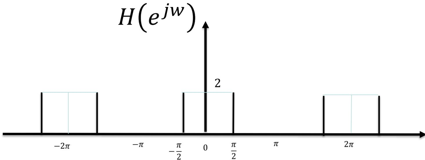
$$h(n) = \frac{1}{2\pi} \int_{-\frac{\pi}{2}}^{\frac{\pi}{2}} H(e^{j\omega}) e^{j\omega n} d\omega = \frac{\sin\left(\frac{n\pi}{2}\right)}{\frac{n\pi}{2}} = S_a\left(\frac{n\pi}{2}\right)$$
