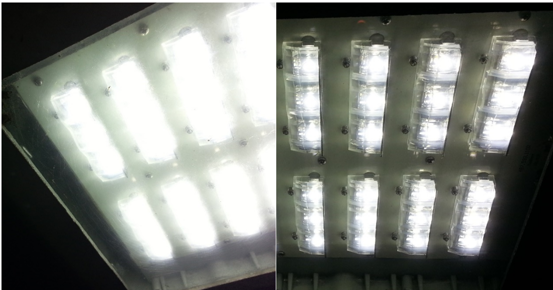
Figure 54. Design J, flat glass over large molded optics, dirty (left), clean (right).
