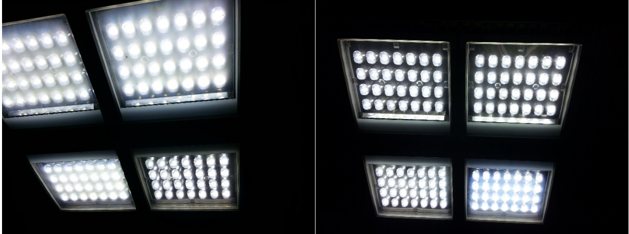
Figure 55. Design K, flat glass optics over individually molded optics, dirty (left), clean (right).
