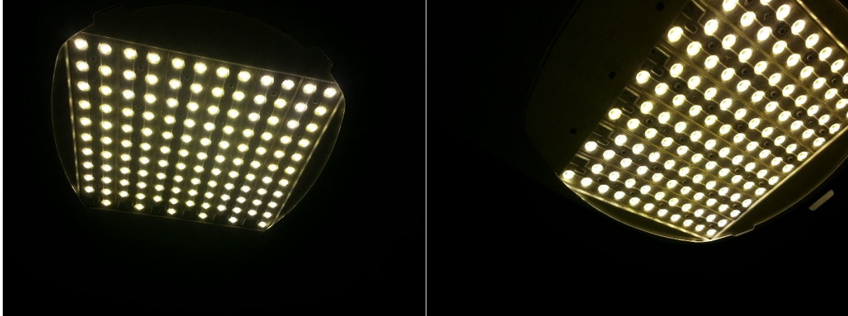
Figure 53. Design G, individual molded plastic optics, dirty (left), clean (right). The photographs do not capture the difference between the dirty and clean very well.
