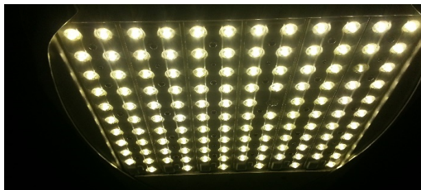
Figure 52. Design G showing failure of one LED unit out of 126.
