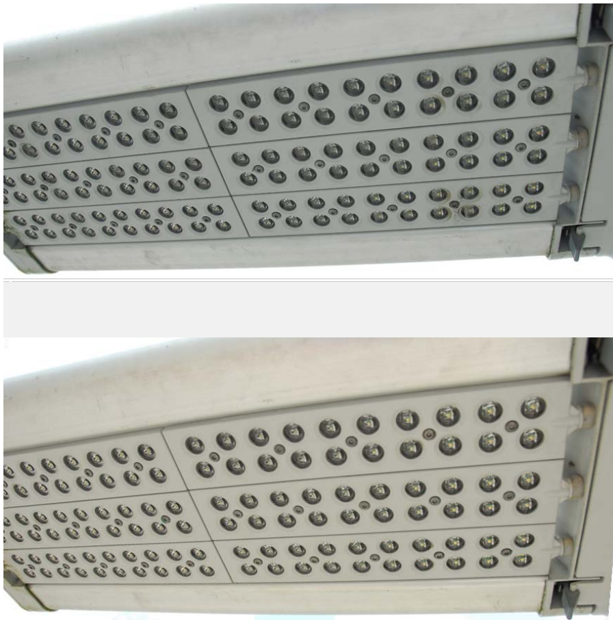
Figure 29. Smart Road LED luminaire before (top) and after (bottom) cleaning with an IPA rag (Cleaning Method 3).
