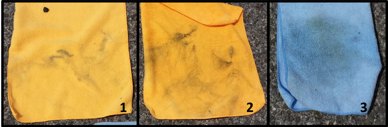
Figure 28. Dirt removed from the luminaires with the first three cleaning methods: (1) dry rag, (2) wet rag, (3) rag with IPA.
