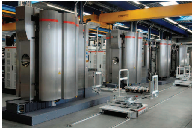
Figure 9.34: Industrial multizone deposition system for the fabrication of DLC coatings for automotive parts and other applications. Each chamber contains six 1.6 m long electrodes. (Courtesy of Hauzer Techno Coatings.)
