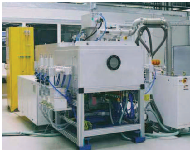
Figure 9.28: Large-area PECVD coating system for the fabrication of barrier and antireflective coatings over an area of up to 55 \text{ cm} \times 55 \text{ cm} . (Courtesy of Roth & Rau.)
