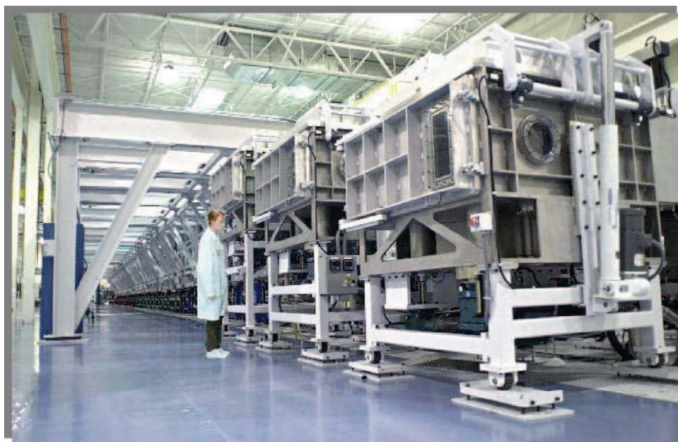
Figure 9.29: Large-area roll-to-roll deposition system for the fabrication of amorphous silicon triple-junction photovoltaic cells. (Courtesy of United Solar Ovonics.)
