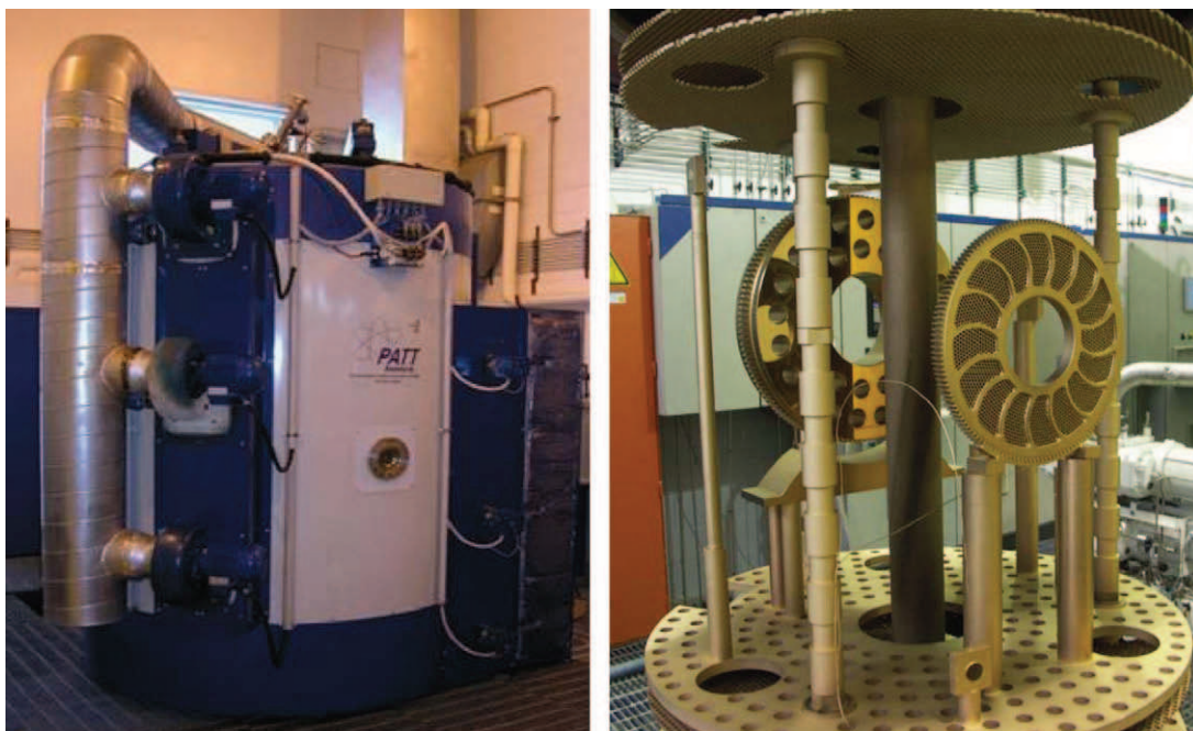
Figure 9.35: Example of a commercial system for the deposition of hard protective coatings. (Courtesy of PATT Technologies Inc.)
