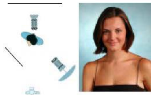
Page 3. Using one head with a brolly and a background light with a honeycomb and a reflector panel
