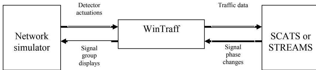
Figure 2.1: Topology of an emulation MSTM for the modelling of adaptive signal control
